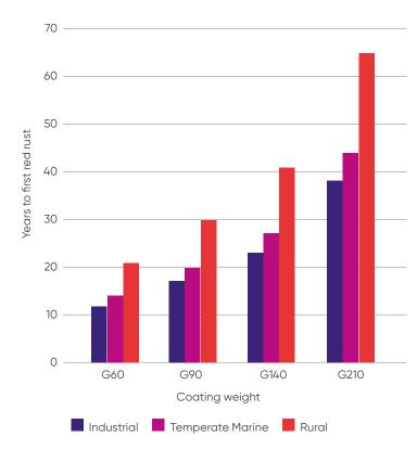
The zinc coating provides galvanic sacrificial cut edge protection to prevent corrosion (rusting) on exposed edges. For these applications, as steel thickness is increased, heavier galvanize coating should be used to ensure sufficient galvanic edge protection for the increased cut edge surface area.
