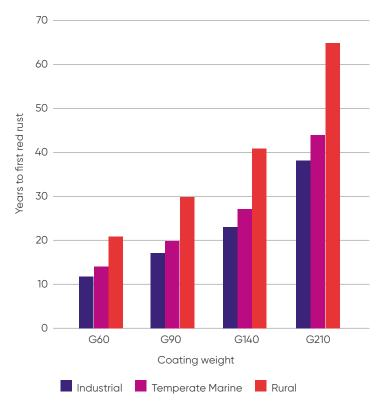
The zinc coating provides galvanic sacrificial cut edge protection to prevent corrosion (rusting) on exposed edges. For these applications, as steel thickness is increased, heavier galvanize coating should be used to ensure sufficient galvanic edge protection for the increased cut edge surface area.
